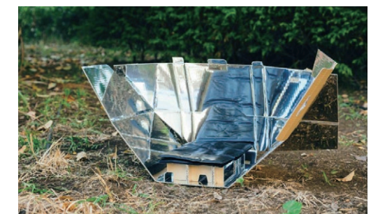
Solar heat is gathered using a solar collector and used as a heat reserve for the mat
