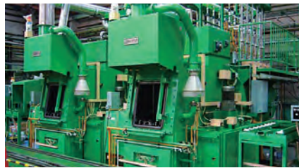
Heat-treatment furnace installed with a single-end radiant-tube burner
