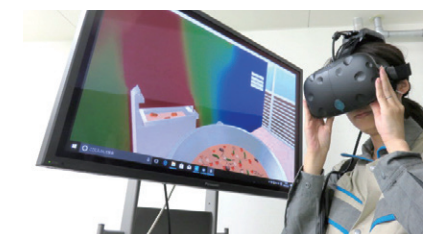
Virtual reality (VR) for checking kitchen temperature distribution
