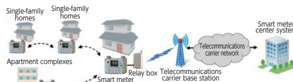
Configuration of the gas smart meter system
